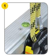
Use level bubble to ensure ladder is at correct angle, and level to terrain accordingly. Adjust TerrainMaster wheels to ensure ladder level.
