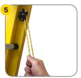
Tension tethers with up to 20Kg of load on each tether.
