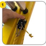
Release tether lever on rear side of ladder and pull rope out.
