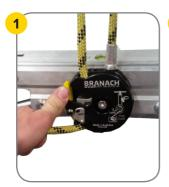
Firmly hold the free end of life-line rope in one hand. Then partially pull out the yellow release lever.
