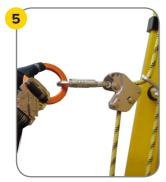
Remove slack in life-line rope by holding the fall-arrest device under the rung hook and pulling the rope line through the fall-arrest device.
