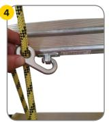
Ascend ladder, once the desired work height on the ladder has been reached, attach the work positioning hook to a rung eyelet above the harness attachment point. Place hook above eyelet and twist in.
