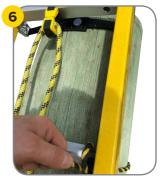
If performing pole work, attach the top-lash to the pole.
