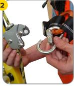
Attach chest harness point to fall-arrest device. Never connect to the fall-arrest device via a lanyard or shock pack as this will increase fall distances and overload the ladder system. The maximum gap between the users' chest and the fall-arrest device should be 30cm.
